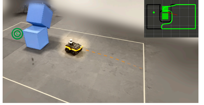
Fig. 4: A snapshot of the Jackal hardware experiment. The robot detects the suddenly fallen obstacle blocking its path. The top-right inset shows the robot’s internal map at the moment of detection; the safe set (green) has not yet been updated to incorporate the new SDF map (black), highlighting the need for rapid, in-the-loop replanning to ensure safety.
